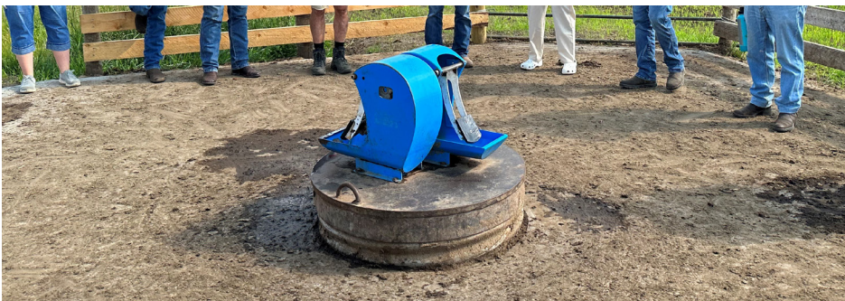
Frost-free nose pump. A year-round watering option that is frost-free without supplemental heat.
